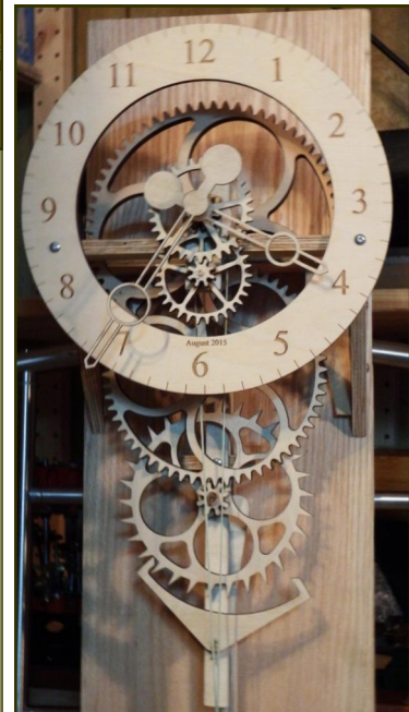
The "Two Paul's" wood works clock with wheels and dial made with a laser cutter
